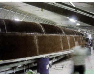
BOTTOM, THE HULL MOULD IS COVERED WITH PRE-PREG CARBON FIBRE BEFORE THE VACUUM BAGS ARE APPLIED TO SQUEEZE THE LAMINATE DOWN. (PICS - JOHN MORRIS)
