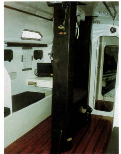
LEFT – THE HM 1300 SWIFTY. RIGHT – THE "HALF CASE" FOR THE LIFT KEEL KEEPS THE INTERIOR OPEN.
