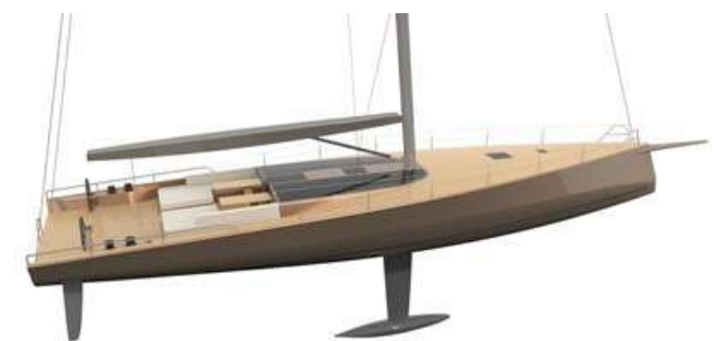
The Baltic 68 Café Racer features flax fibre construction and many other innovative materials.
