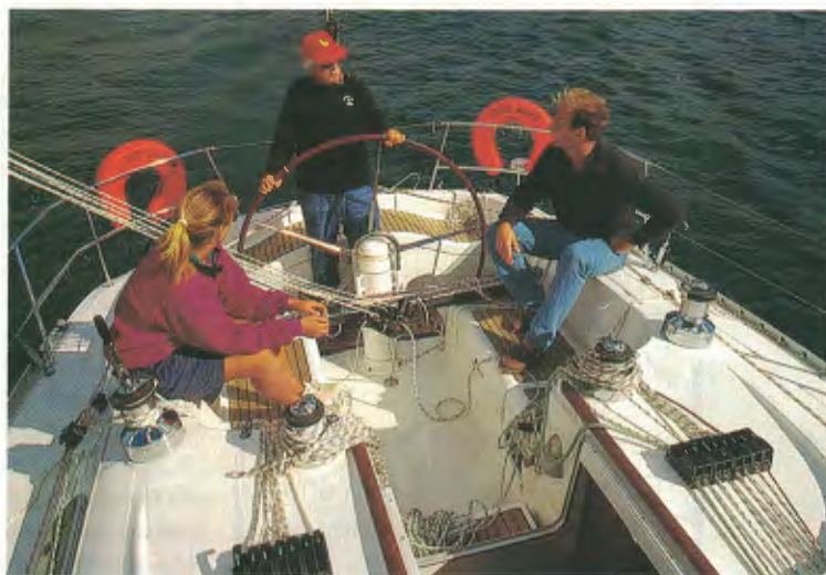
Looking aft to the large cockpit of the Beneteau 42sf, Lorita Maria . IMS cruiser/racer has traveller splitting the cockpit.
