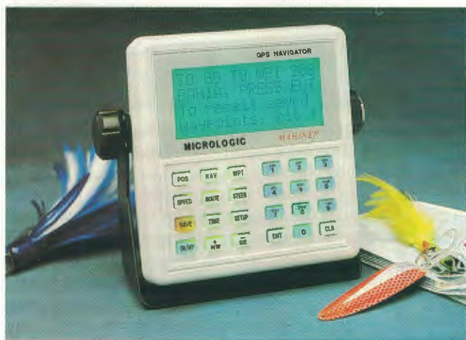
Micrologic Mariner GPS is an affordable unit suited to nav station mounting
