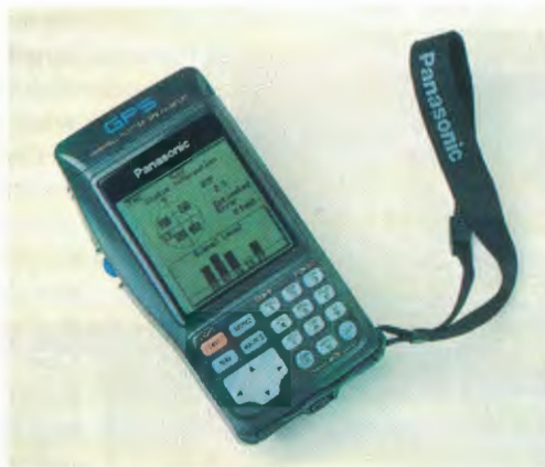
Left: This new handheld from Panasonic combines plotter functions with normal GPS functions
