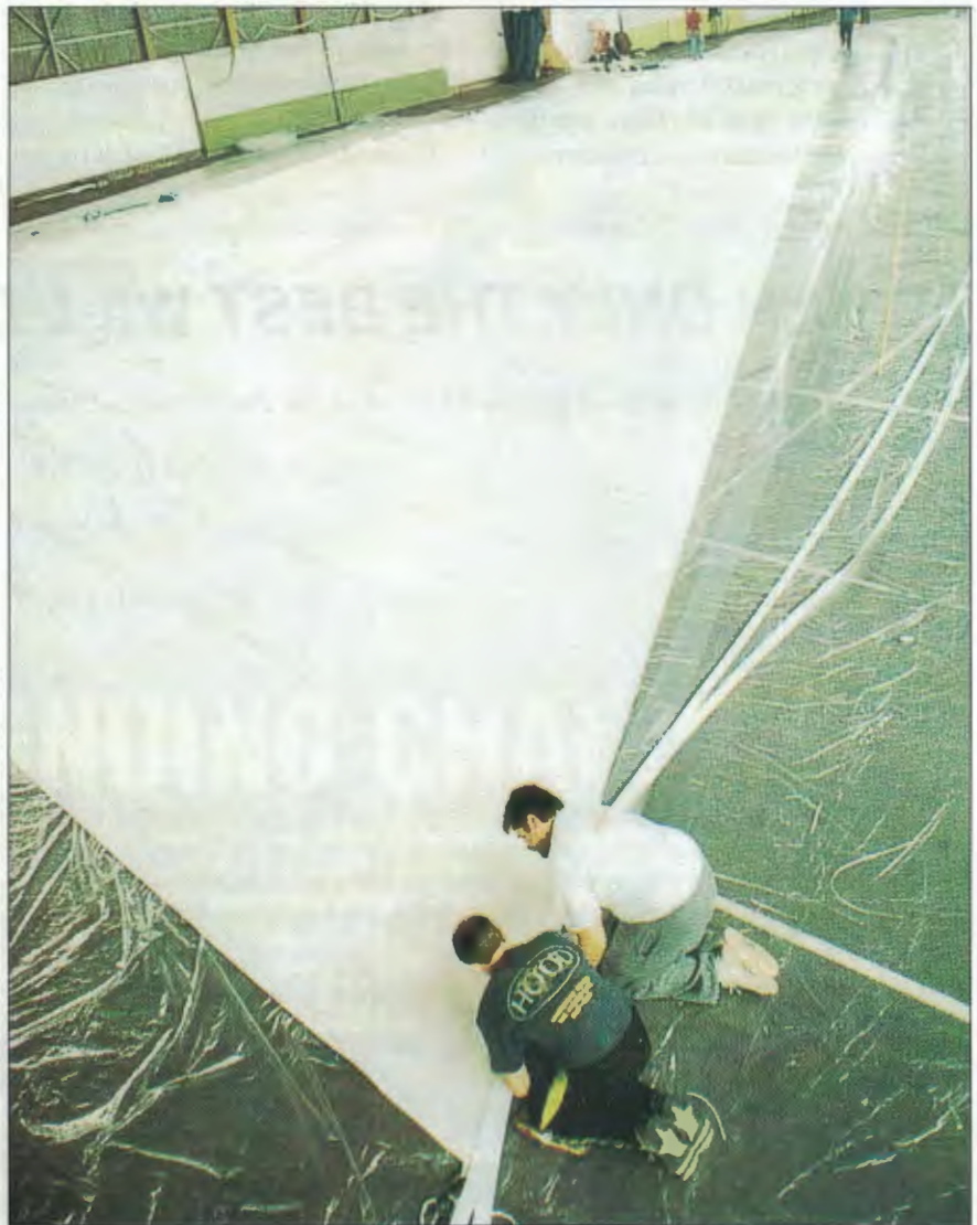
Below: Hood's new Vectran sailcloth ... four tennis courts were hired to lay out the Vectran Yankee for the ketch Thalia
