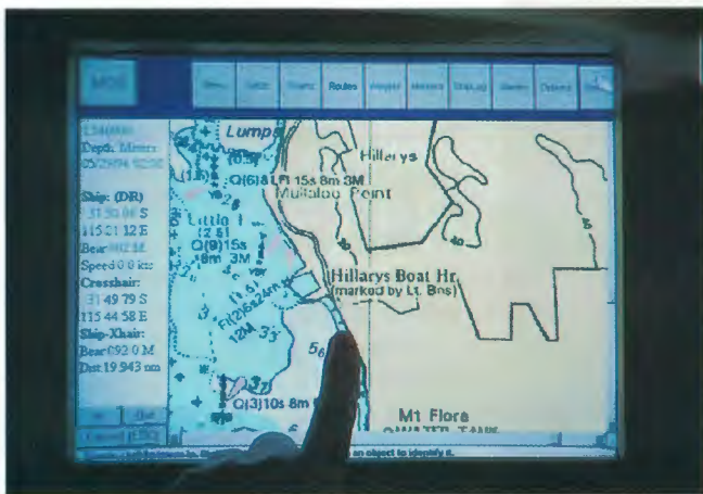
Above left: PCs with special Touch Screens, in which the finger replaces the mouse, are increasingly popular with commercial fishermen. This Micro Mariner navigation program is using an authorised scan of an Australian Chart, distributed on floppy disk. Above right: Waypoints, routes, tracks, and GPS positions etc are superimposed on the ARCS chart by the navigation software.
