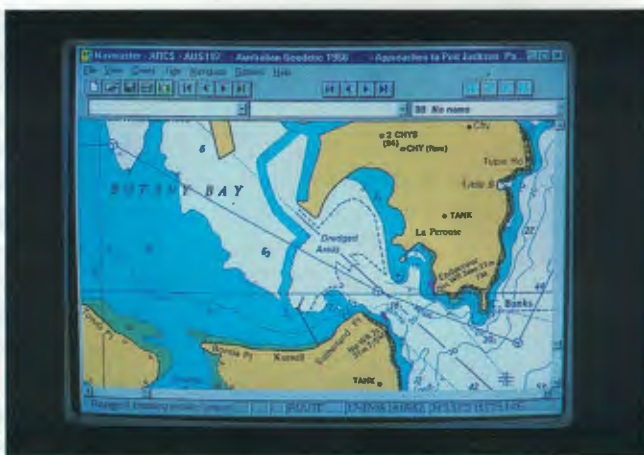
Above left: PCs with special Touch Screens, in which the finger replaces the mouse, are increasingly popular with commercial fishermen. This Micro Mariner navigation program is using an authorised scan of an Australian Chart, distributed on floppy disk. Above right: Waypoints, routes, tracks, and GPS positions etc are superimposed on the ARCS chart by the navigation software.
