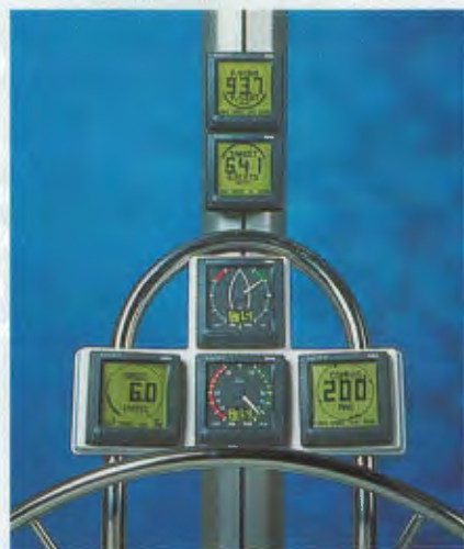
The Corus RACE performance system now includes the new Corus RACE600, providing target speed, % performance, optimum VMG and adjusted time at a glance.
