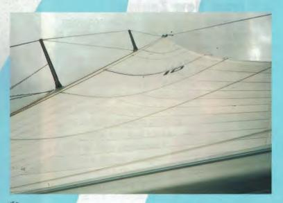
sail as it furls, so that stays efficient and fast when reefed. In designing a Furl-boom mainsail, Hood Sailmakers shape it like a conventional mainsail and use full length battens. This helps prolong the life of the sail and help maintain a more efficient shape.
