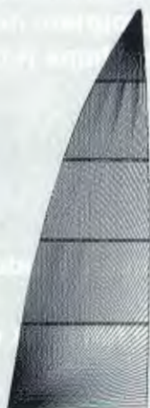
The yarn array for a D-4 mainsail shows how the denier count can be varied in each section.
