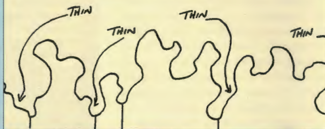
The thinnest (lowest) points indicate the true protection level
