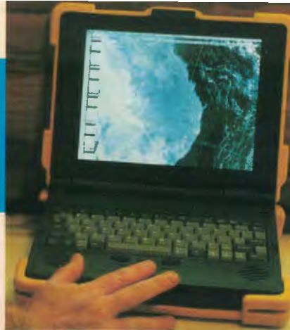
Image of the Australian east coast received real time via a Quorum Voyager receiver, and displayed on this Rocky notebook computer.
