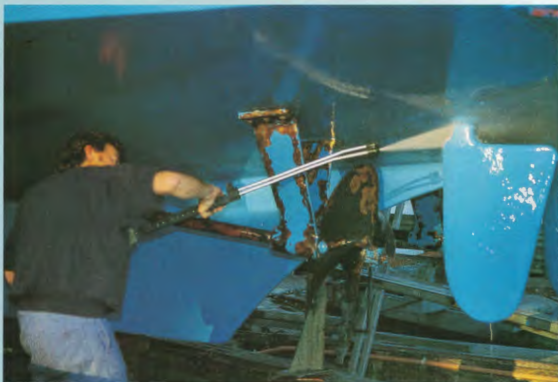
"Gurni-ing" high pressure water removal of marine growth and slime before the antifouling begins. (Pic - Theresa Biggelaar)
