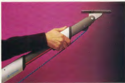
The Spinlock small Powervang, designed for performance cruisers and one-design racers under 30 foot LOA.
