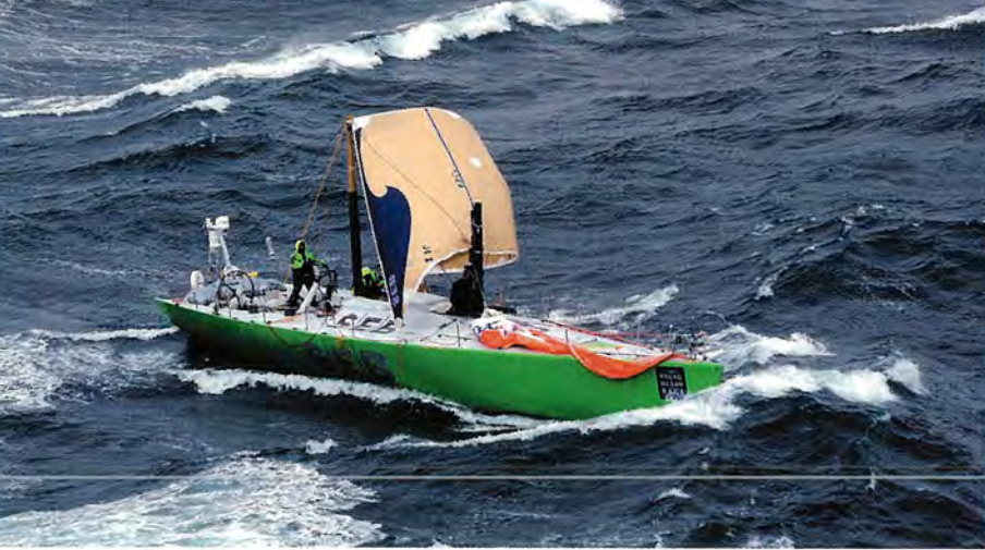
SEB sails on under jury rig after being dismasted in the Southern Ocean Photo – Rick Tomlinson
