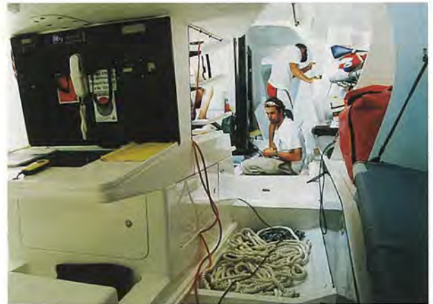
The saloon navigation station is located aft of the companionway in the bare layout below decks for what is essentially a racing boat
