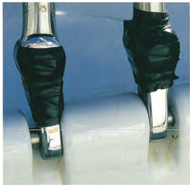
Composite chainplates to prevent water drips
