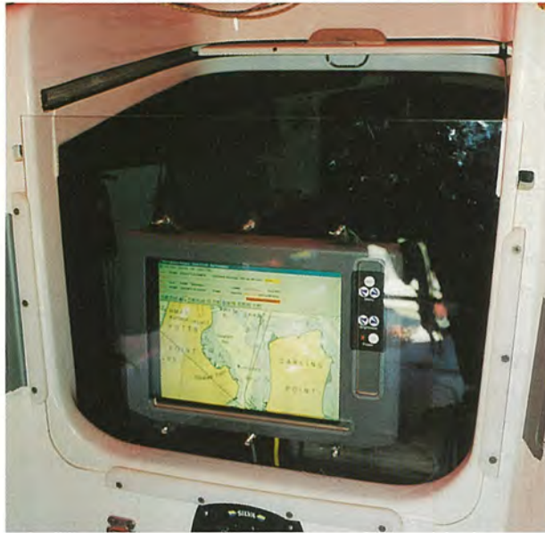
Top: A nav station, from far left – the barometer, switchboard, AM/FM radio / CD player, VHF radio, GPS, laptop and HF radio Above: The slave screen in Krakatoa's companion way
