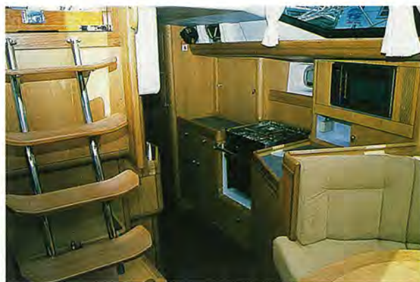
The galley is in the walkway between the saloon and the master cabin aft. The sink is on the inboard side and the narrow gap is ideal for safety Photo – Barry Tranter
