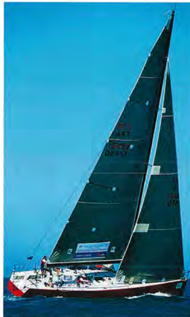
Carbon fibre is believed to be better at holding sail shape than aramid alone Photo – Cheryll Kerr, courtesy North Sails
