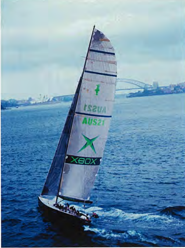
As a result of the trickle-down technology from the America's Cup, more and more carbon-fibre sails are being used at club-racing level Photo – Cheryll Kerr, courtesy North Sails
