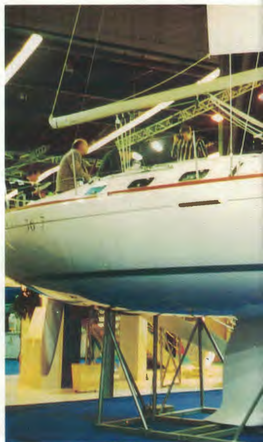
Above: Pleasing hull lines of the Beneteau 36 s7, created by French naval architect Jean Berret indicate the power of the boat. This boat has the 1.85m draft cast iron bulb keel.
