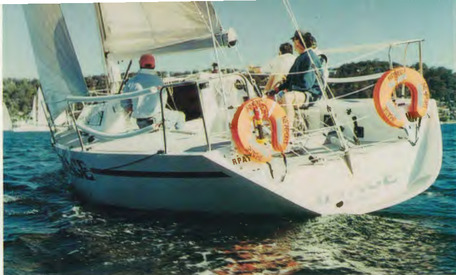
New cleaner deck has no cockpit coamings as well as extended counter stern.
