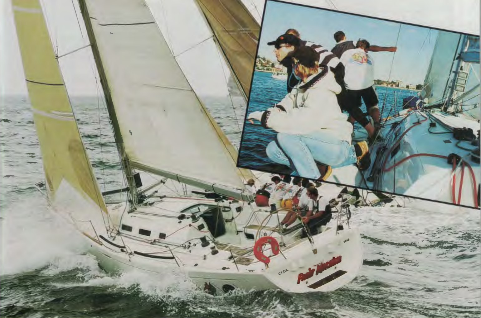
Deck layout of the Beneteau First 40.7, Fruit Machine , is almost stock. It works well as it is and the crew prefer to hone their sailing techniques rather than chop the boat about. This photograph was taken from near the helm. Because the 40.7 is a cruiser/racer the wheel is small and sited well aft, so the helmsman doesn't have a great view of the headsail luff.
