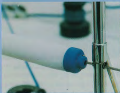
Neat arrangement of the Titan Ends Caps which extend the durability of lifeline cushions.
