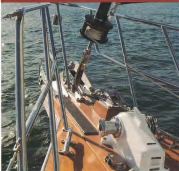
ABOVE: Cockpit provides great security BELOW: Muir reversible anchor windlass
