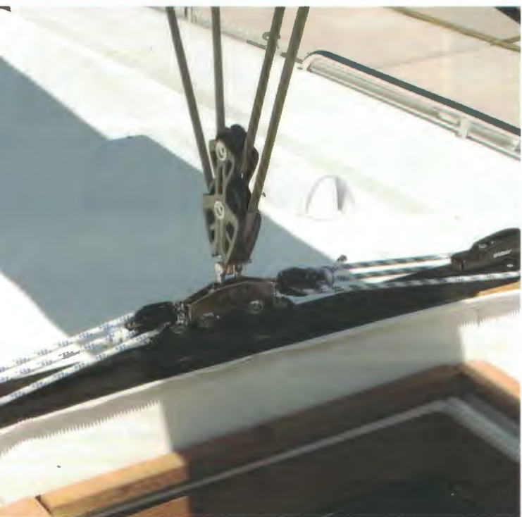
Control lines are led aft beneath deck mouldings
