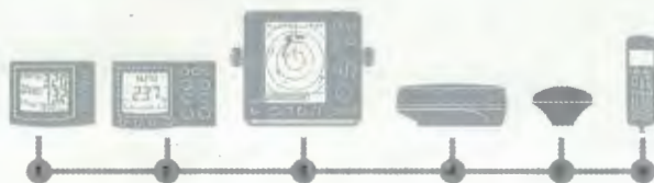
1.ST290 2.ST7001 Autopilot 3.RL80C 4. 24" Radome 5.Raystar 120 GPS 6.Ray 230E
