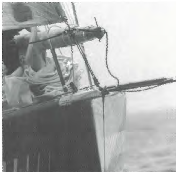
AMERICA'S Cup Challenger finalist New Zealand midway through a gybe, bowsprit downhaul still tensioning luff of gennaker. This was ruled illegal by both the Louis Vuitton Cup and America's Cup Juries – but an incident that the Kiwis claimed lasted only for eight seconds yet cost them a race win. (Pic – Pickthall Picture Library)
