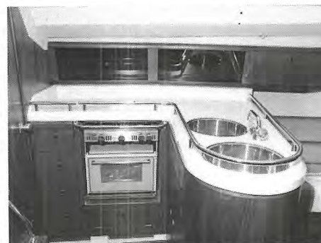
TOP: Before launching picture of Sigma 35 shows clean lines of hull, moderately deep keel, but quite deep rudder. CENTRE: Main saloon with galley to port, navigation area to starboard and large settee berths. BOTTOM: Galley layout with twin sinks, gimballed stove and large GRP work surface. (Pics – Robert Chapman)
