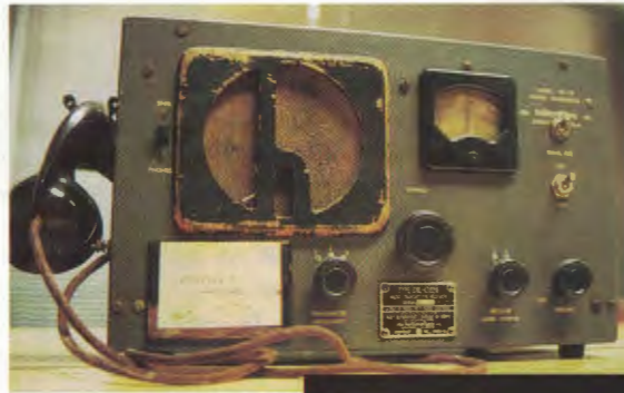
The old and the new...a two-band 12 volt US Navy HF transmitter/receiver in common use during World War II, and communications in the satellite age. The United States has already introduced legislation to require all marine radio equipment sold in the US after 1997 to be fitted with GMDSS-automated facilities.
