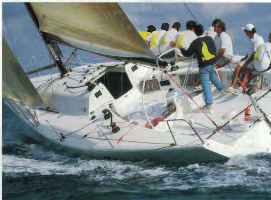
Spacious and simple cockpit layout of the Farr 40 One Design, uncluttered by having no backstay runners. (Pic- Peter McGowan).
