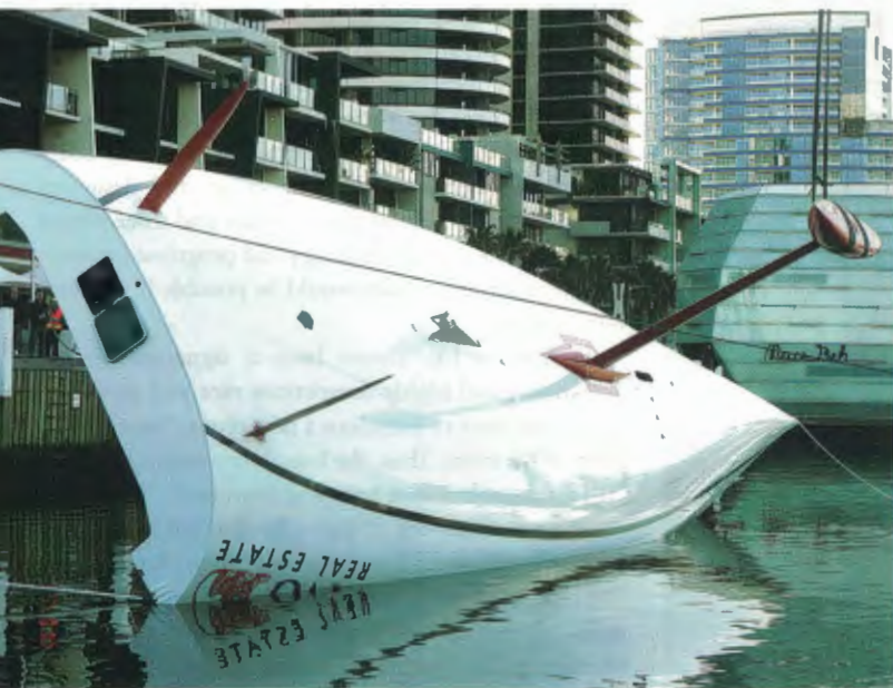
Testing the righting moment of the Premier Challenge boat PHOTO: Courtesy of Premier Challenge
