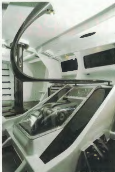
The transparent cover reveals the workings of the hydraulic ram that moves the canting keel PHOTO: Edward Rowe
